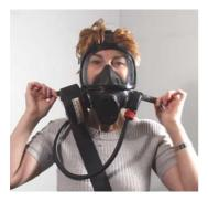
Tighten the straps in sequence: bottom, side then top. DO NOT over-tighten as this distorts the faceseal.
