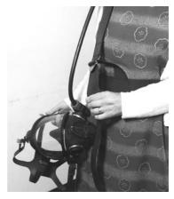
Fasten the waistbelt and adjust the shoulder strap for a comfortable fit.
