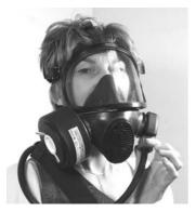
Open the bypass switch and check that there is a steady flow of air into the facemask.
