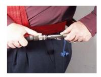
Push the airline couplings together and pull back the CEN collar to disconnect the airline hose
