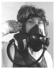
Check that the bypass switch is in the closed position and inhale sharply to activate the first breath mechanism.
