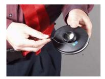
Check that the cord from the filter cover is around the filter connector. Check that the filter is in-date (see filter label).
