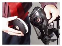
Check that the filter O-ring is in place and in good condition. Screw the filter to the facemask.
