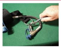
Check there is no damage or excess wear in the bandolier and that the shackle is securely attached to the D-ring. If necessary tighten the shackle nut.
