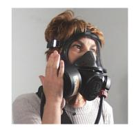
Press the filter seal with the palm of the hand to seal the filter inlet, and inhale. Hold your breath for 10 seconds. Check that the facemask pulls on to the face and does not pull away during the 10 seconds.
