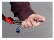
Use a thumb to seal the airline coupling.
