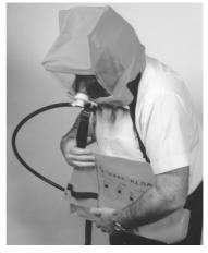
Check that there is a steady flow of air into the hood.
