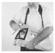
Hold the bag and pull the flap to withdraw the firing pin. Listen for air flowing into the hood.
