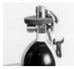
Fit the firing pin and quick-fire strap.
