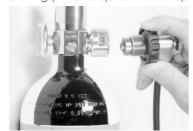
Fit 200 bar G5/8 pattern charging connector to the charging adaptor.
