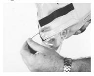
Check that the anti-tamper tags are in place and unbroken.
