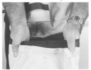
Place the palms of the hands together and insert through the rubber neck seal. Open the hands to open the hood.
