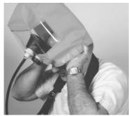
Hold the hood with the neck seal over the crown of the head and pull the hood down over the head until the neck seal is around the neck. Check that clothing or hair is not trapped in the neck seal.
